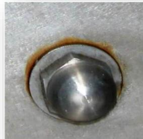
This specific corrosion problem can be avoided with preventive actions using as a protection Zinc-o-fix® product. This product has been used for many years in the production of vehicles and means of public transport, and for their maintenance. In the specific case, and in all corrosion cases due to the coupling of metals with fastening elements, the problem is solved introducing between the elements a shape created according to the client's need.
